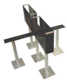
This elevated plus-maze a sturdy apparatus frequently used to measure anxiety levels in rodents and to screen potential anxiolytic drugs. There is no raised edge or margin along the open arms, and the ends of the closed arms are also open. This design allows for modification and upgrading as needed. What we have achieved with this plus maze is simplicity, affordability and ruggedness for manual anxiety protocol needs.
